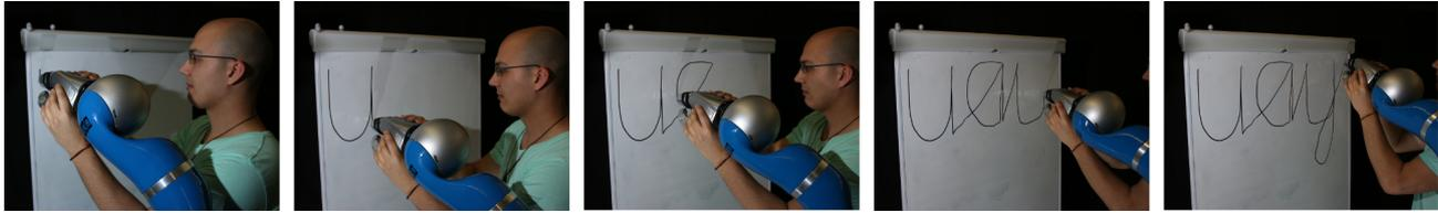
(a) While holding a pen, the robot was demonstrated writing trajectories on a white board using kinesthetic teaching.
