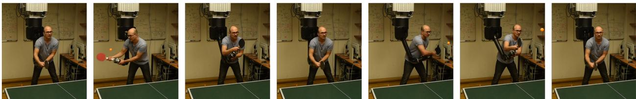
**Figure 14.** Kinesthetic teaching of the barrett wam robot platform for the table tennis task. While one person throws table tennis balls towards the robot, another person moves the robot manually in order to return the balls. During the teaching all seven joints are recorded for the subsequent segmentation.
